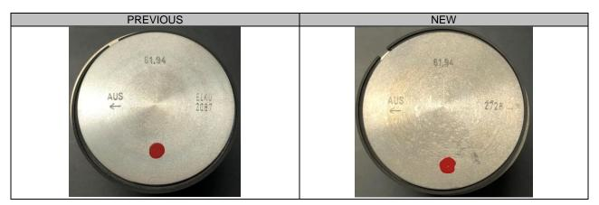
Additionally, the color on the first few batches of new pistons can appear slightly darker. The different surface color is caused by the new cutting plates. The surface will eventually get shinier due to the natural cutting edge wear. This effect is typical for pistons made from an alloy with 25 % silicon. This has no impact on quality or functionality; it is purely cosmetic.
